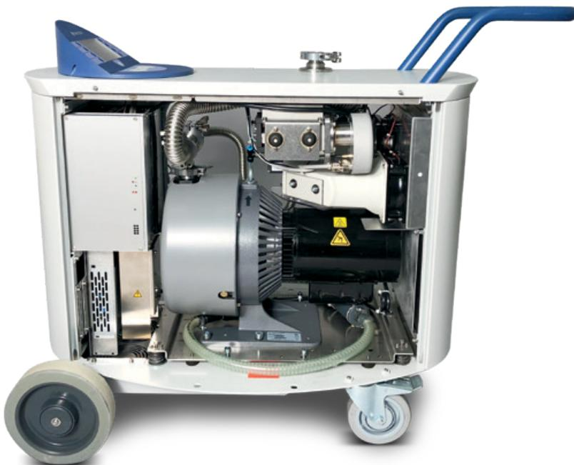
$10^{-12}$  mbar-l/s combined with reasonable short pump down and response time. The compact design provides high maneuverability allowing easy access to maintenance areas with restricted space. The selectable background suppression (I-ZERO) enables continuous leak testing within at least two decades lower than existing background levels.
